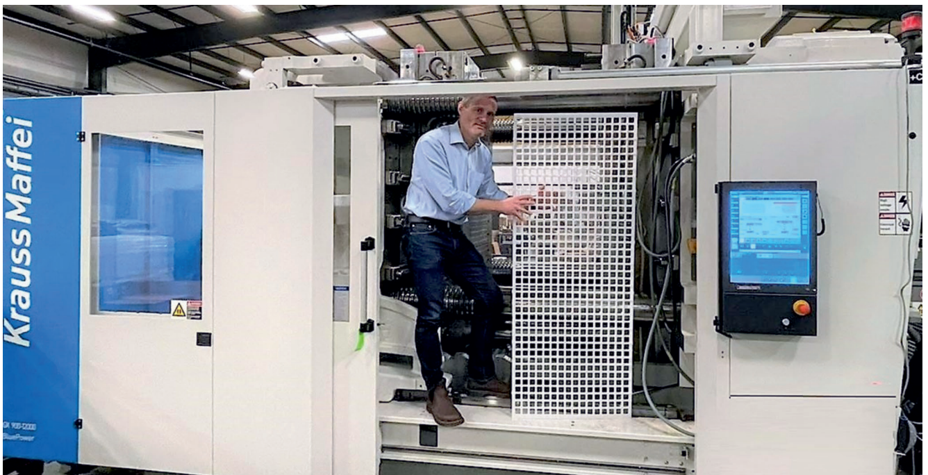
Sebastian Lotzin, CEO of Barku's U.S. subsidiary, with floor grate (3250 g) in the 10,000-kN injection molding machine that makes the part © Barku
